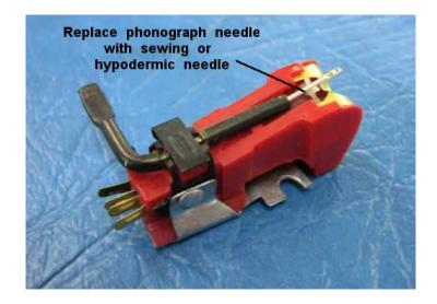
You can make an exceptionally sensitive displacement transducer using a crystal or ceramic phonograph cartridge; these are still widely available from sources on the web for about \$20. In place of the phonograph needle, which is a replaceable component, insert a 2- to 3-inch (50 – 75mm) sewing or hypodermic needle. Attach the end of the needle to the object to be monitored. You may need to experiment to determine which cartridge output terminals give the best signal out to the Model 2991.
