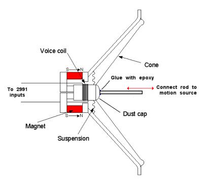
To measure small amounts of linear displacement (up to a few millimeters), connect the Model 2991 to the voice coil terminals of an inexpensive loudspeaker. Then glue one end of a rigid stick or rod to the center of the loudspeaker (the domed paper or plastic dust cap). Attach the other end to the moving object to be monitored. This transducer gives excellent results in measuring linear displacement due to the change in voice coil inductance.
