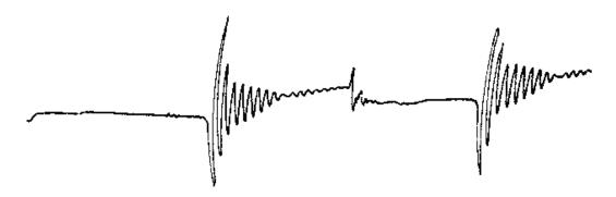
Damped oscillations recorded with two needle electrodes, separated by about 0.25" (6mm), that projected into a saline stream flowing at a constant rate. Damped oscillations were recorded from the Model 2991 output when the flow was stopped abruptly with a pair of hemostats.
