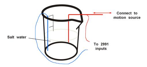
Other linear displacement transducers have been made with two stiff wires suspended in a beaker filled with salt water. One wire (blue above) is fixed; the other (red) is attached to the moving object. Start with just a pinch of table salt, and add until the resistance between the wires at maximum distance is no more than about 2000 ohms.
