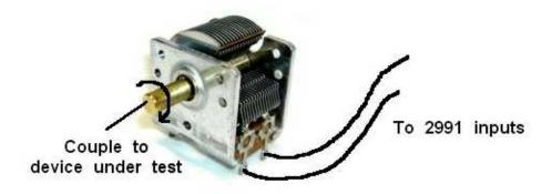
An ordinary 365pF variable capacitor, of the type once used to tune AM (medium-wave) radio receivers, may be used to measure torque or rotational displacement. Simply couple the rotating shaft of the capacitor to the rotating device to be measured. The Model 2991 is sensitive to a capacitance range between about 200pF and 1,000pF.
