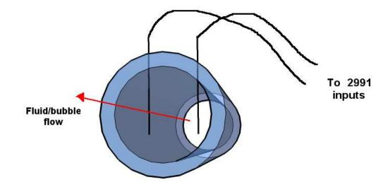
To use the Model 2991 as a bubble sensor, arrange two needle electrodes across from one another in the fluid stream. (If the stream flows through soft plastic tubing, you can just push the needles through the tubing.) Any bubble passing between the electrodes will cause an impedance change that can be detected by the Model 2991.
