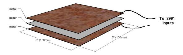
Two metal sheets, each about 6" x 6" (15cm x 15cm) and separated by a piece of paper, make a functional "quick and dirty" capacitor for displacement or tension measurements.
