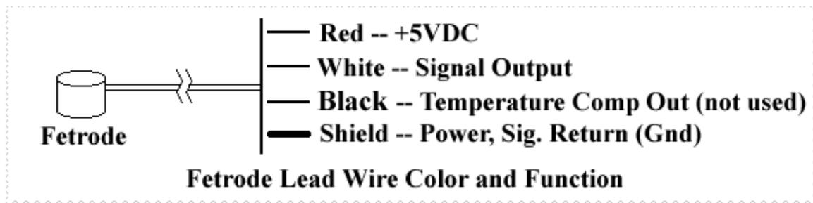
The RED wire should be connected to a +5-volt DC supply. The voltage should be well decoupled using appropriate capacitors and should be stable, preferably regulated. Supply voltages higher than +5 volts can be used -- up to +15 volts -- but may introduce additional noise.
